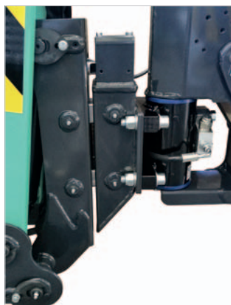
Compact jib group with load cell and basket rotation system.
